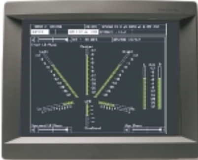
One of many types of audio displays offered by the VTM-300G, CineSound® surround sound monitoring.
