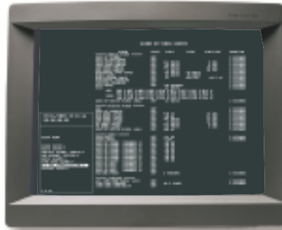
VTM-300G alarm settings alarm screen, a snap shot of all alarms that can be recalled with the press of the display button.
