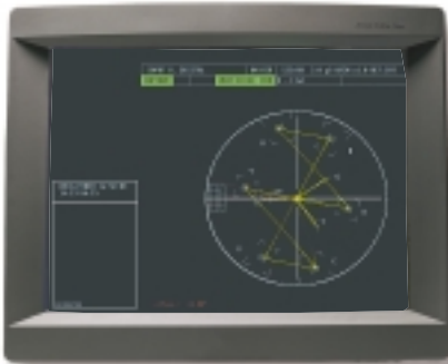
Vector display with Reference and Delta cursors used to measure color phase.
