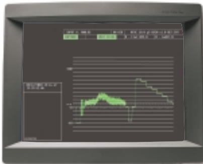
Two video inputs displayed in A/B Parade. Two waveforms, A-Flat Filter, B-Low Pass Filter, and different lines selected.
