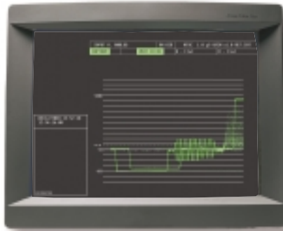
Two Video Inputs Displayed in A/B Overlay. Note Timing difference.
